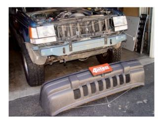
2. Mount brackets with tube extensions facing the frame. They are used to offset the brackets when mounting the bumper. Leave brackets loose until bumper is in position.
